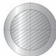
circular thread cross section
