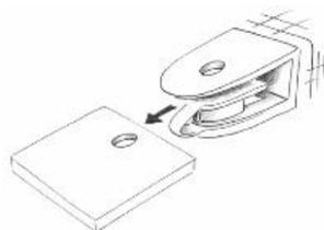
A novel fastening element that can be used for assembly on varying thicknesses of components, realized through an axially movable center part; the actual boss. The boss is kept in its position by two opposed spring elements, thus the EASYboss® V does not cause rattling noises under vibration nor will the fastening element fall off.
