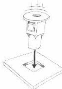
The EJOT SQUAREboss is a tailor-made fastening element. In combination with the DELTA PT® screw it allows an economic and safe joint. Assembly in the substructure takes place by manual pushing through in assembly direction.
